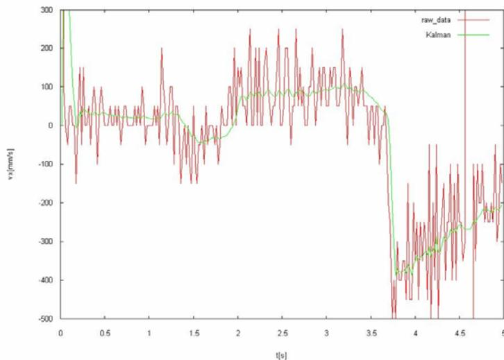
Fig. 5 Noise decrease by using Kalman filter
