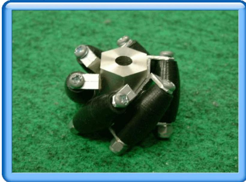
**Fig. 1 The mecanum-wheel**
